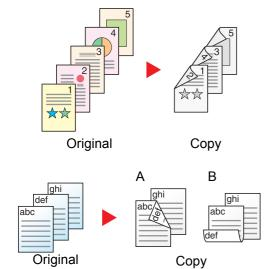
Produces two-sided copies from one-sided originals. In case of an odd number of originals, the back side of the last copy will be blank.
