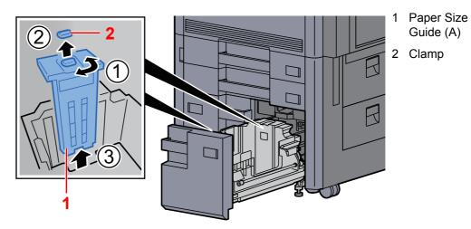
Insert the Paper Size Guide (A) into the slot (bottom of cassette) for the paper size to be used.
