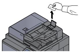
Clean the slit glass surface and the reading guide.
